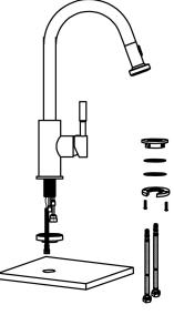
brace, U-shape washer onto the thread tube(pipe). Tighten the lock nut securely.
