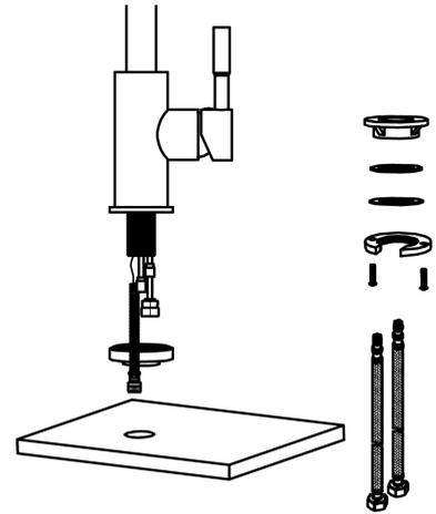
The rubber O-Ring must be installed under the faucet body and on the sink or counter surface.
