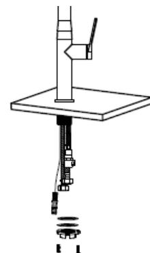
brace, U-shape washer onto the thread tube(pipe). Tighten the lock nut securely.
