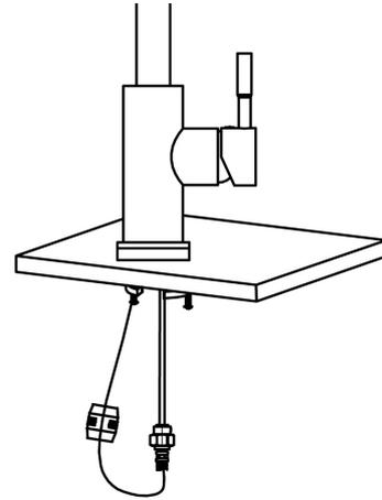
8. Connect the water supply lines with the faucet body. The cold water line is on the right and the hot water line is on the left. Then connect the cold and hot water lines with the angle valve.
